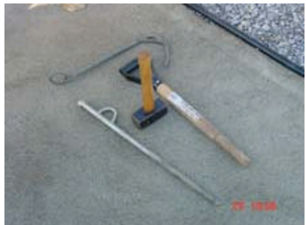
Mooring pins and lump hammer
