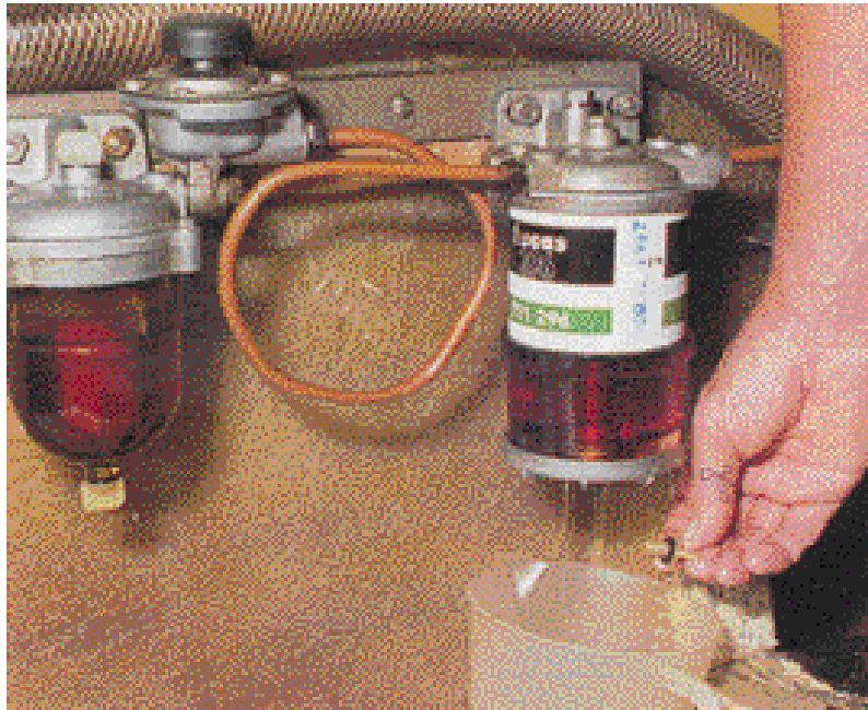
Fuel filter, water trap and sediment bowl with drain
